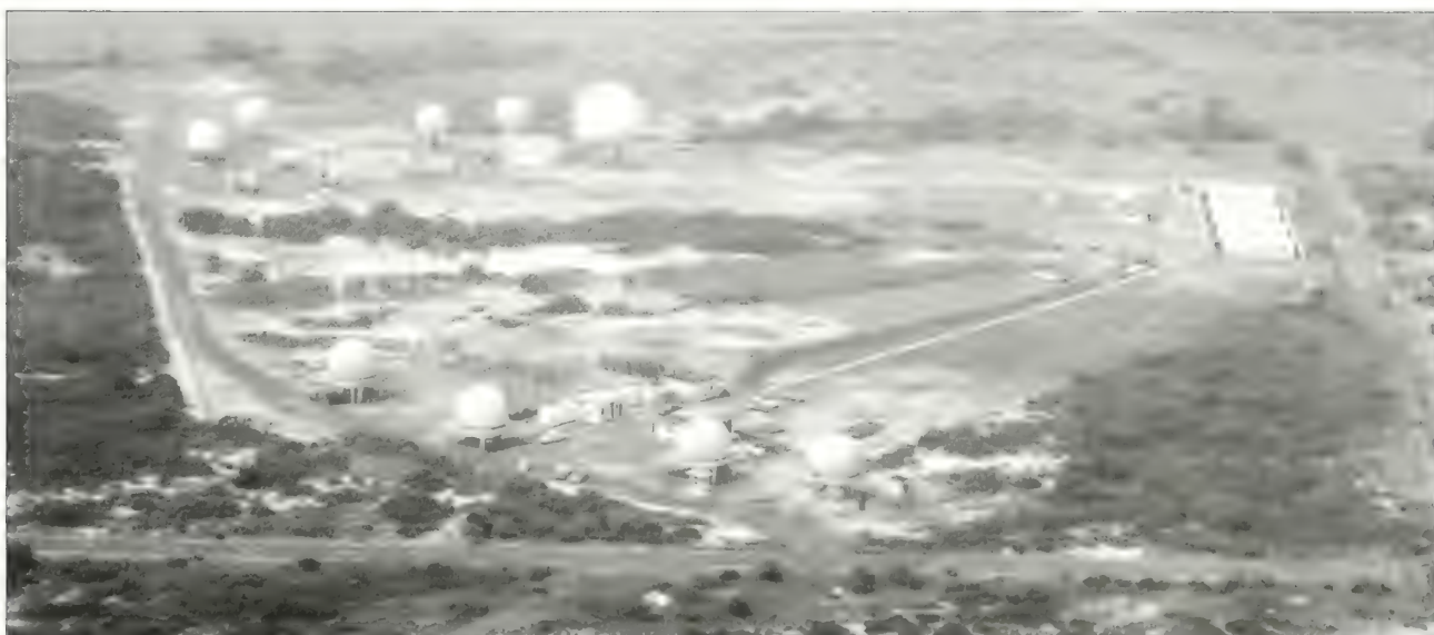
Figure 5.97. Oblique aerial view, NIKE radar site, circa 1962. In this photograph Control Area #2 is in the foreground with Control Area #1 in the background and the Ready Barracks to the right. In addition to the thirty-foot fire break inside the perimeter fence, most of the vegetation on the site was strictly managed except for a wedge-shaped area in the center (GATE 20818).
